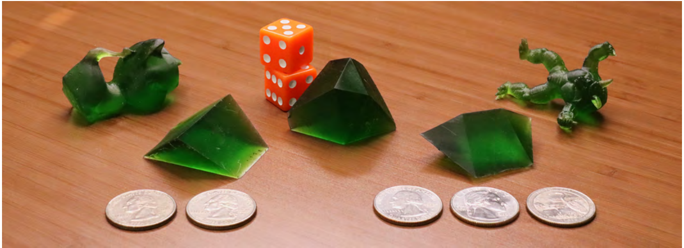
Fig. 1. We introduce a geometric model for the resting equilibria of rigid bodies. This model supports fast differential evaluation, enabling tasks such as the inverse design of dice with prescribed probabilities. As shown in the photograph above, we design single dice that capture the statistics of other objects such as the sum of a pair of ordinary dice (middle), or the number of heads from flipping two or three fair coins (front). We can also deform nonconvex shapes such that their stable configurations exhibit dice-like probabilities; here, the kitten and armadillo models both have just three stable configurations with equal probabilities.
