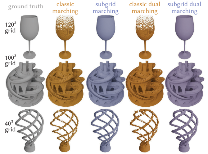
Fig. 18. Even at very low resolutions, our subgrid approach better preserves surface topology—which can have a profound impact on visual fidelity.
